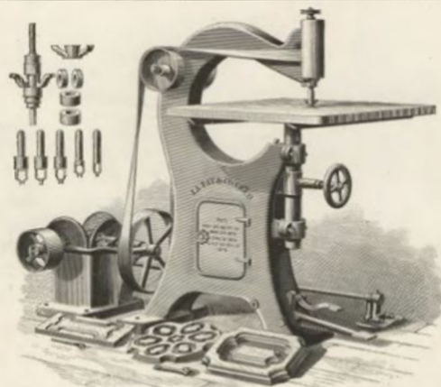
Patent Carving and Edge-Molding Machine. With Patent Friction Reversing Countershaft.
